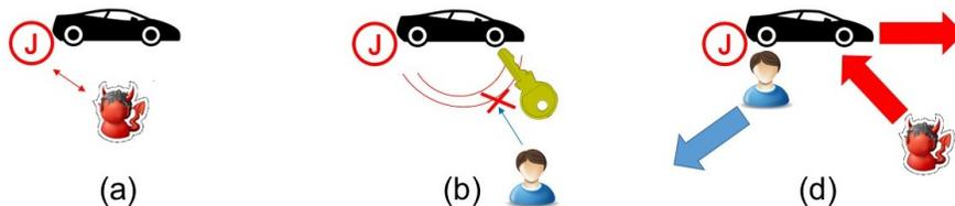
**Fig. 1.** The attack is performed in a sequence of 3 steps: (a) Jammer set-up and activation, (b) Jamming the communication between the user and the car and forcing the user to use the mechanical key, and finally (c) when the user leaves the car unattended, the adversary hijacks the car.
